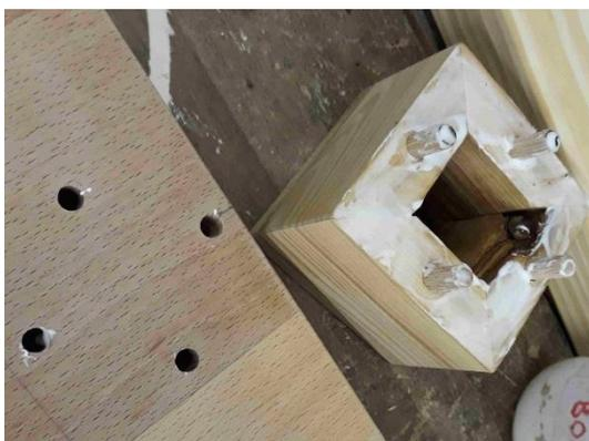
8. Measure, mark out and drill holes in the middle of each side for wood dowels.
